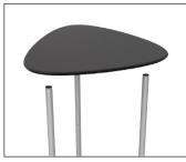
3.Place counter top onto poles.Tap down with hand to secure.
